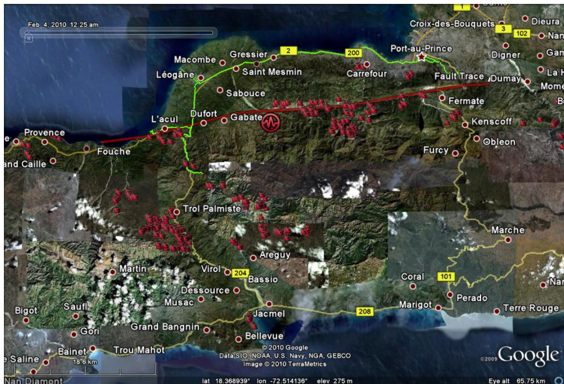
Figure 9.1 Landslides (red) identified by aerial imagery by Ed Harp of the USGS. Green track is route traveled by GEER team on day of landslide investigation. (Imagery from Google Earth)
